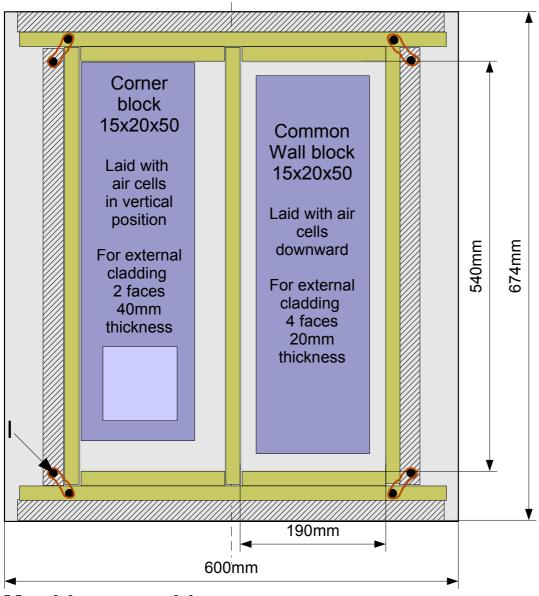
A mould to transform concrete blocks into reconstituted cut stones
